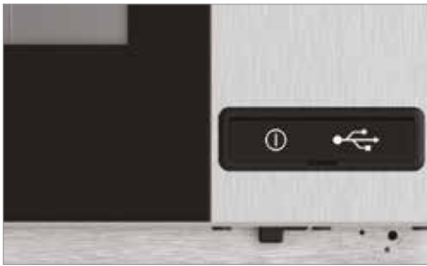
USB PORT FOR UPLOAD/DOWNLOAD OF DATA
